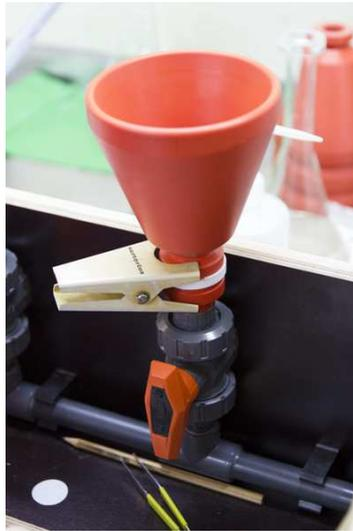
Figure 8.3: Set Up of Filtration, the filter is between the red cone and the 'Fritte'.
