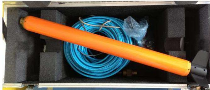
Figure 6.3: Explorer Magnetometer Towfish
