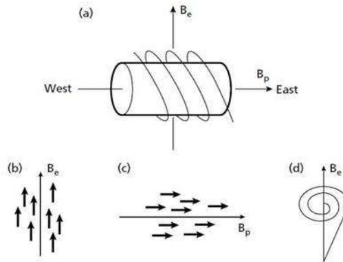
Figure 6.4: Proton Magnetometer principle
