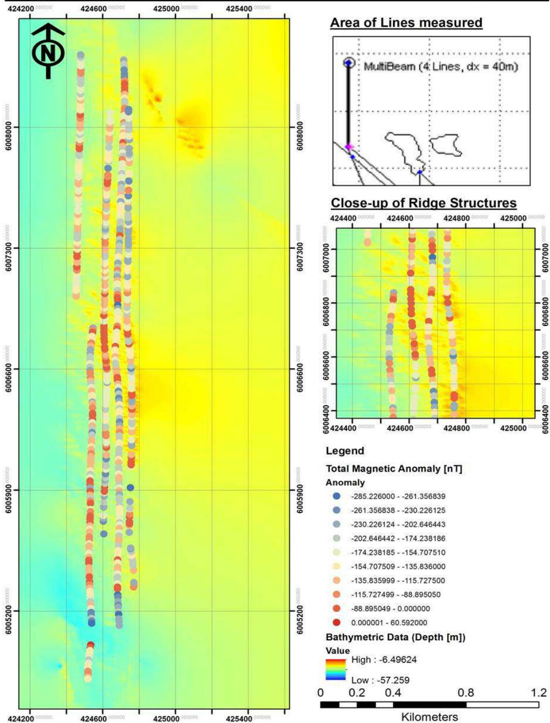
Figure 6.8: Magnetic Anomaly Map plotted over Bathymetric data measured North-West of Helgoland
