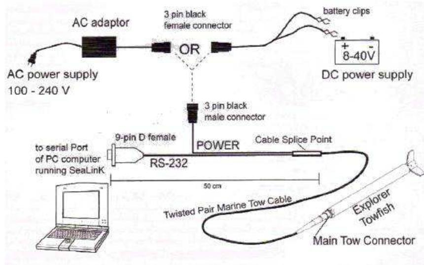
Figure 6.6: Data collection Set-Up
