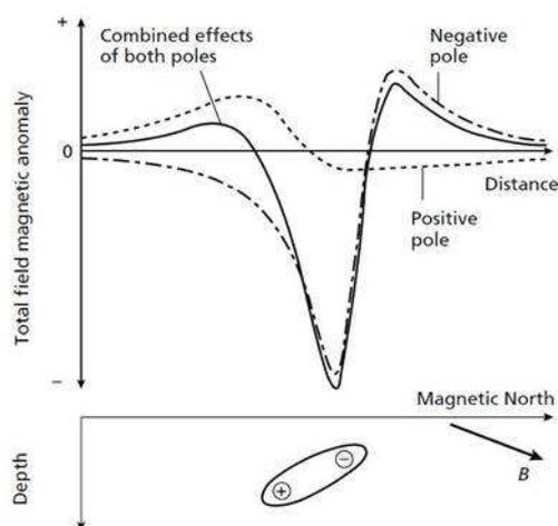
Figure 6.2: Total magnetic field anomaly of an elongated body
