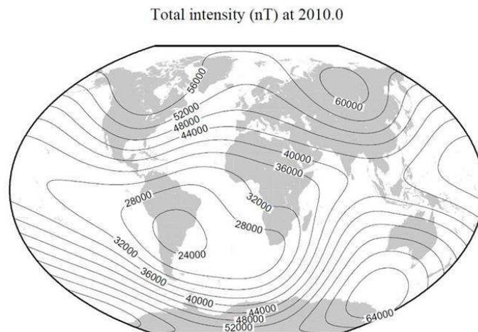
Figure 6.1: Contour map of total intensity (nT) at 2010.0
